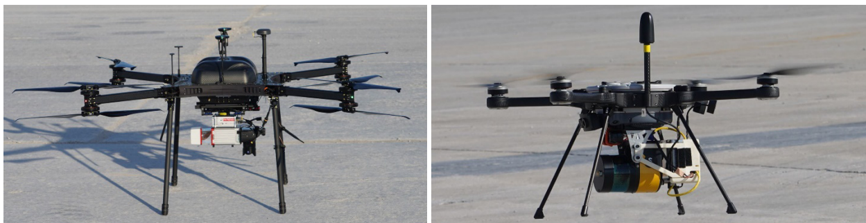
Figure 10: Harris H8X UAS with miniVUX2 LiDAR (left), SkyRaider UAS with Surveyor Ultra (right).
